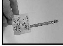
Remove pencil and pour contents into the Reagent Chamber tapping the bottom of the pouch to dislodge all the powder.
