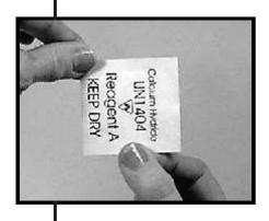
Hold the sealed calcium hydride packet by one side and flick the opposite side of the packet several times with your finger to cause the granules to flow to the side of the pouch which is facing down.
