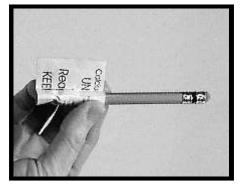
Roll pouch tightly around the pencil. You now have a cylindrical opening from which to pour the calcium hydride.
