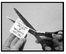
Using a pair of scissors, cut the top of the packet off, just above the words, "Calcium Hydride".
