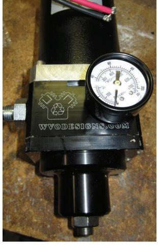
Add included pressure gauge to 1/8"NPT ports.
