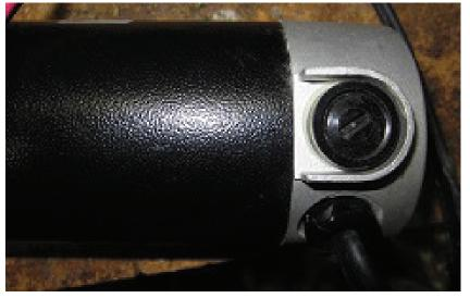
Mount horizontally, with brushes horizontal to the road and wire conduit nut facing down to reduce risk of water contamination.
