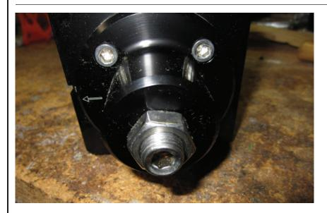
Prime the pump and then make adjustments to the variable adjustment screw on the bottom of the pump. Losen larger lock-bolt to make adjustment to the smaller screw. Tighten pressure adjustment screw clockwise to increase pressure. Pumps are initally set around 20 PSI. There must be some tension on the screw to insure 15+ PSI, otherwise the pump won't prime. Pump won't regulate less than 15psi.
